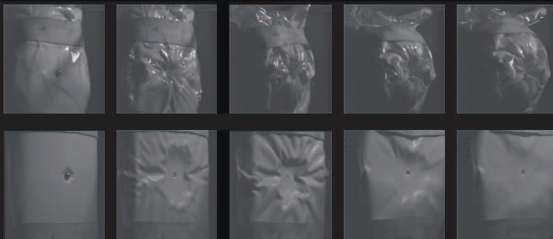
An illustration of the differing impacts of a bullet on traditional armour (top) and BAE Systems' Liquid Armour (bottom).
